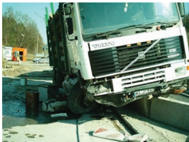
Fig 10. The truck carrying logs hit and crashed through the barrier and left the carriageway of the bridge over river Nemunas (courtesy of "Lietuvos Rytas")
