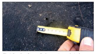
Fig 4. Samples of geotextile damages (puncturing) whose mass per unit area is  $110 \text{ g/m}^2$  laid between the subgrade and the frost blanket course
