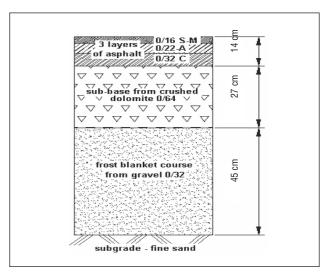
Fig 1. A typical road pavement structure
