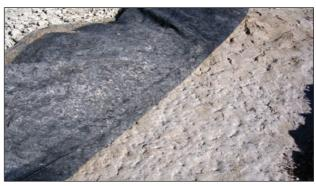
Fig 9. The performance of the road pavement layer separation by geotextile after uncovering the layers of the second test section of the pavement structure – the separation of the frost blanket course and the sub-base
