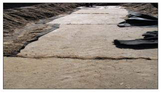
**Fig 8.** The performance of the road pavement layer separation by geotextile after uncovering the layers of the first test section of the pavement structure – the separation of the subgrade and the frost blanket course
