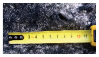
**Fig 5.** Samples of geotextile damages (puncturing) whose mass per unit area is  $130 \text{ g/m}^2$  (laid between the frost blanket course and the sub-base of the pavement)
