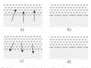
**Fig 2.** Processes active in the layers of the road structure and their prevention by a separation geotextile: a) fine particles of soil migrate into a more porous frost blanket course, b) the migration process of fine soil particles has been terminated, c) large aggregate particles migrate into a weaker layer, d) the migration process of large particles has been terminated
