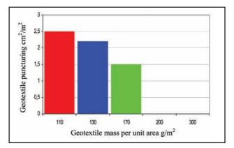
Fig 6. The total area of geotextile punctures  $\mathrm{cm}^2 \ \mathrm{per} \ \mathrm{m}^2$  in the first test section
