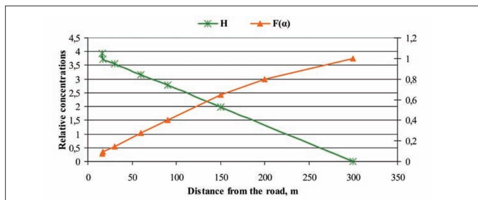
Fig 4. The graphical view of the alteration of the height of pollutant cloud ( $H(x) = 2R - h$ ) receding from the freeway above the ground surface and the probability distribution function  $F(x)$
