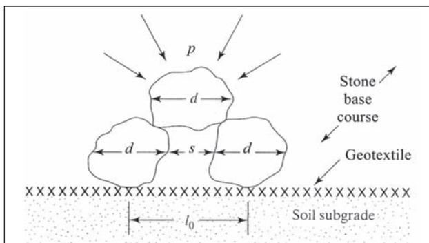
Fig 1. Geotextile being subjected to tensile stress as surface pressure is applied [12]
