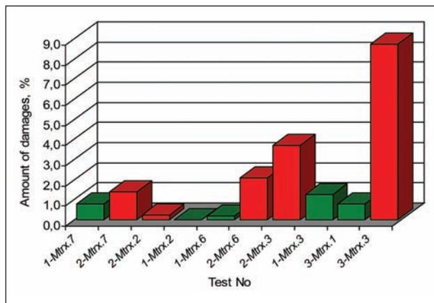
Fig 8. Mean values of geotextiles damage area (GTX1 in green, GTX2 in red)
