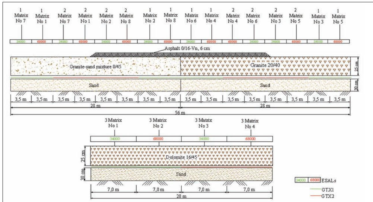
**Fig 2.** The longitudinal section of the test sections
