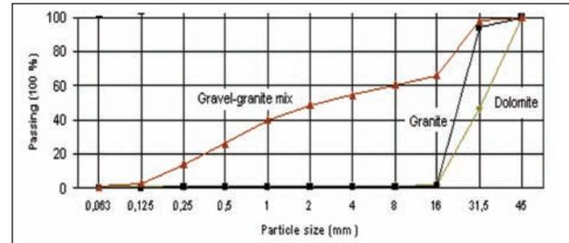
**Fig 3.** Particle size distributions of sub-base materials
