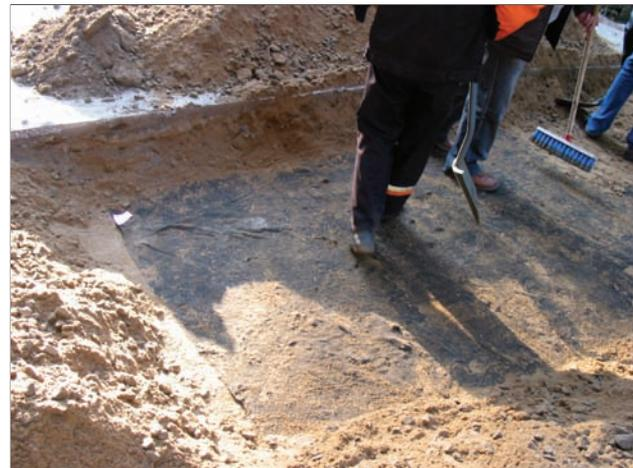
Fig 6. Excavation of geotextiles in the test sections
