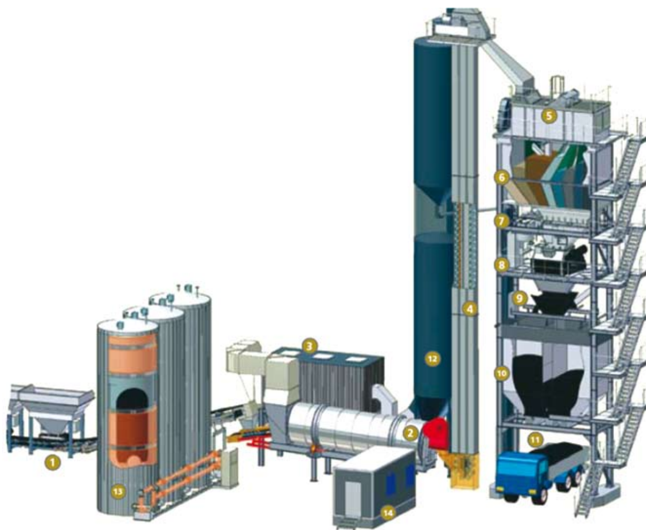
Fig. 1. Construction of batch-type asphalt mixing plant (AMP): 1 – cold feed with integrated collector belt; 2 – drying drum with burner; 3 – filter-type dust collector with centrifugal force coarse dust separator; 4 – chain elevator; 5 – hot screen with bypass changeover flap; 6 – hot aggregate silo with 6 mineral compartments plus a bypass; 7 – weighing platform with scales for mineral materials, imported fillers, reclaimed dust, bitumen and special materials; 8 – mixing platform twin-shaft paddle mixer; 9 – movable hopper, optional horizontal skip; 10 – hot mix silo; 11 – truck loading; 12 – silo tower for reclaimed dust and imported filler; 13 – electrically heated bitumen tank installation; 14 – command container with control system (Available from Internet: < http://www.ammann-group.ch/content/documents/d200404051516458690.pdf > [accessed 2008, May])
