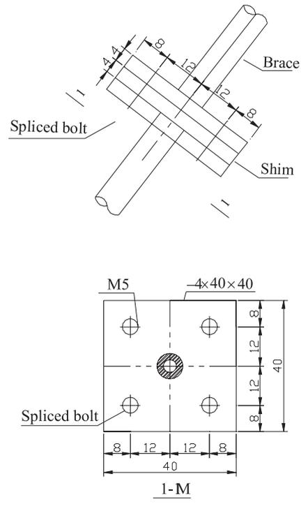
Fig 2. Internal structure of damage simulation position: a – spliced connection; b – cross-section
