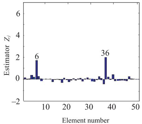
Fig 11. Damage estimator for case 6
