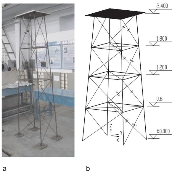
Fig 1. Experimental model of platform: a – real structure; b – FEM structure
