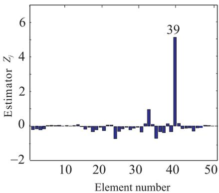
Fig 8. Damage estimator for case 3
