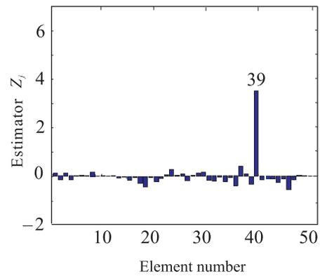
Fig 9. Damage estimator for case 4
