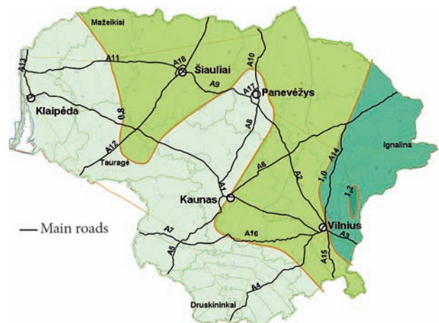
Fig. 3. Distribution of the max depth of frozen ground in the territory of Lithuania based on RWIS data
