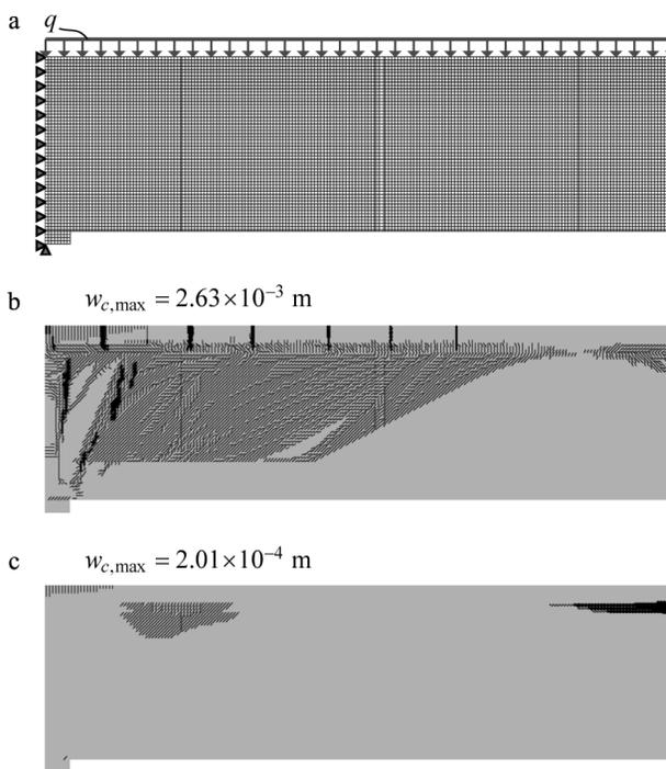
Fig. 8. FEM of the bridge segment (a) and the crack pattern predicted without (b) and with (b) pre-stressing
