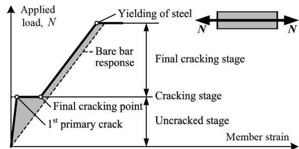
Fig. 2. Idealised loading-deformation response of RC member
