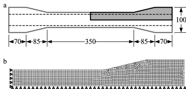
**Fig. 4.** Geometrical parameters of the test specimen (a) and FE mesh of the model (b)
