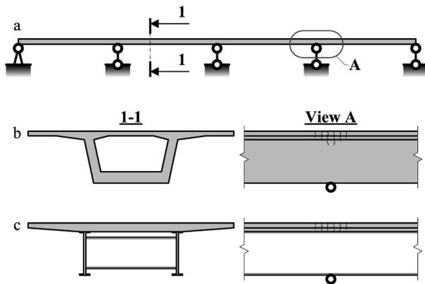
Fig. 1. Sketch of a continuous bridge (a); cracking pattern of concrete (b) and composite (c) sections
