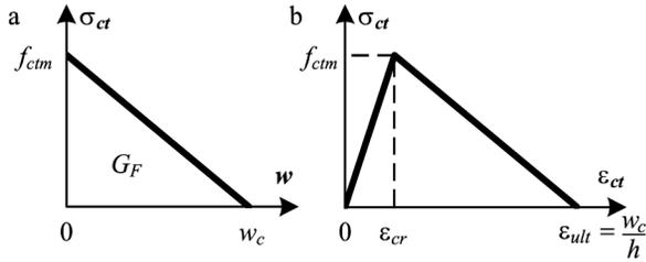
Fig. 5. Tension-stiffening models based on stress-crack width (a) and average stress-strain (b) relationships
