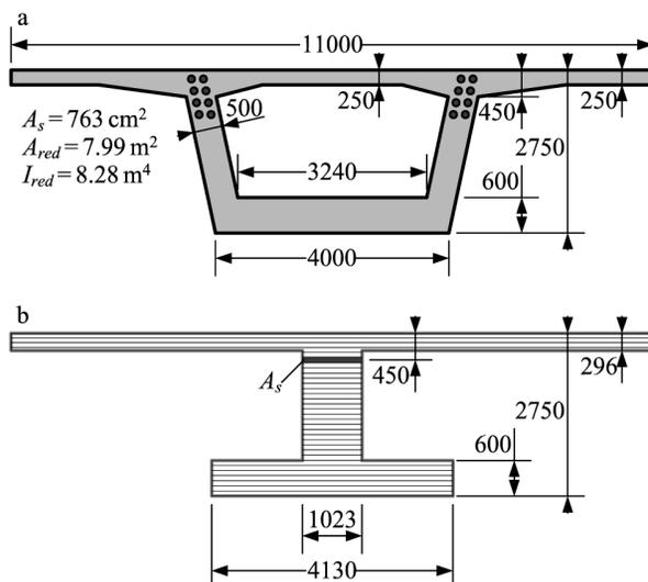
Fig. 7. Box girder cross-section (a) and its Layer model (b)
