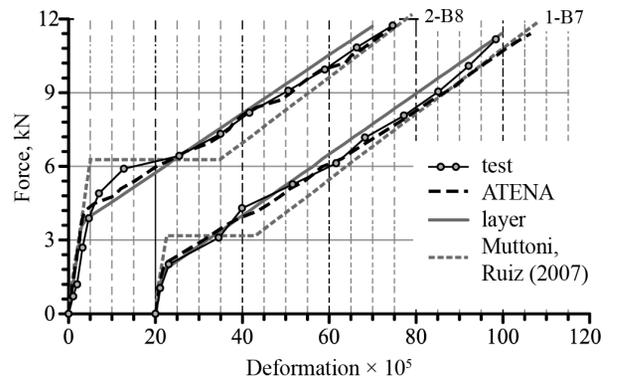
Fig. 6. Predicted deformations of the test members
