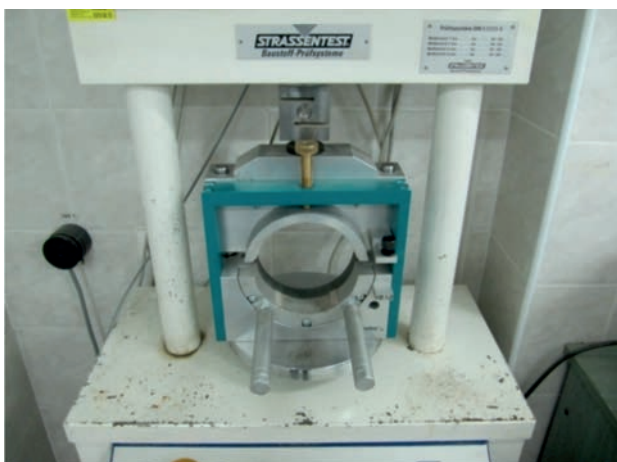
Fig. 2. Asphalt layers shearing mould fixed in the Marshall press
