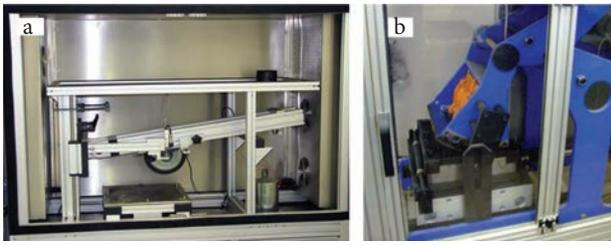
Fig. 3. Test setup for (a) rutting test and (b) slab compaction
