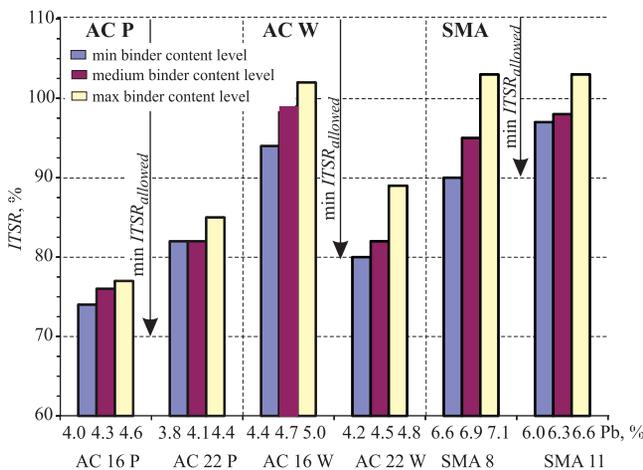
Fig. 6. Test comparison for indirect tensile strength ratio (ITSR)
