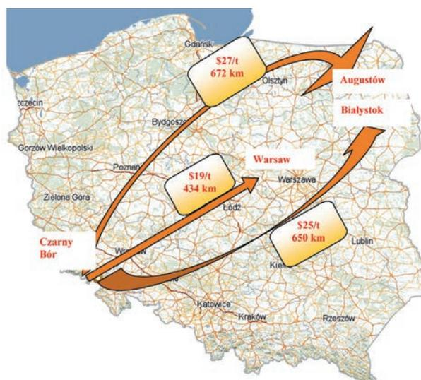
Fig. 8. Comparison of hauling price and distance for aggregates from south of Poland
