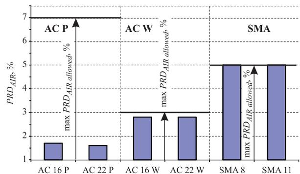
Fig. 7. Comparison of proportional rutting depth values
