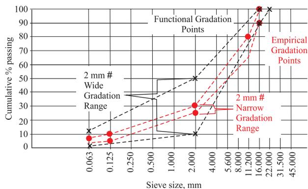
Fig. 2. Comparison gradation points for empirical and functional asphalt mixtures designing method for binder course dense mixture
