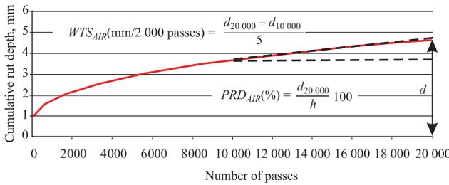
Fig. 4. Typical rutting test results
