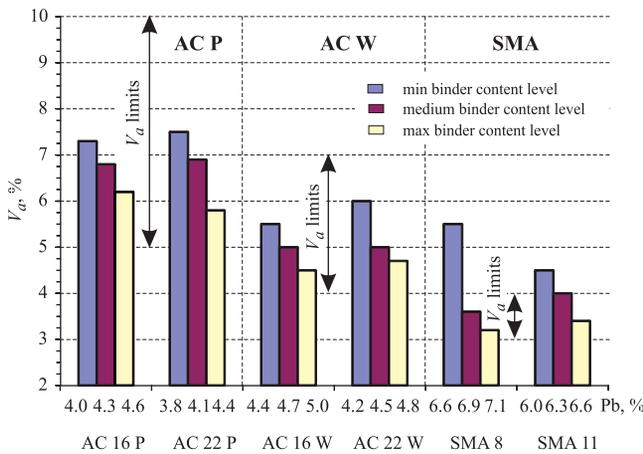
Fig. 5. Air voids determination for different mixes and binder contents
