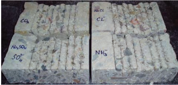
Fig. 2. Selected samples of construction concretes cut in the overpressure vessel by a high-pressure generated water jet
