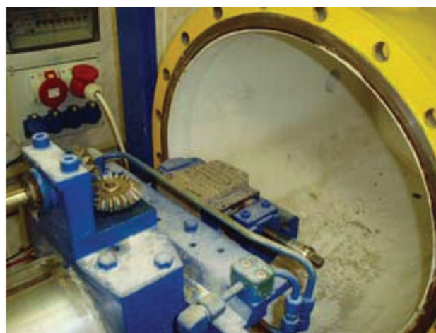
Fig. 1. Support with a sample in front of the pressure vessel
