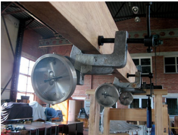
Fig. 9. Maksimov's gauge with the accuracy of 0.1 mm to measure the vertical displacements of the nodal points
