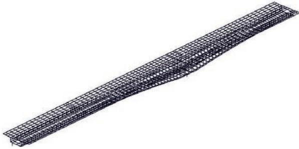
Fig. 10. The space-frame lattice model of half bridge
