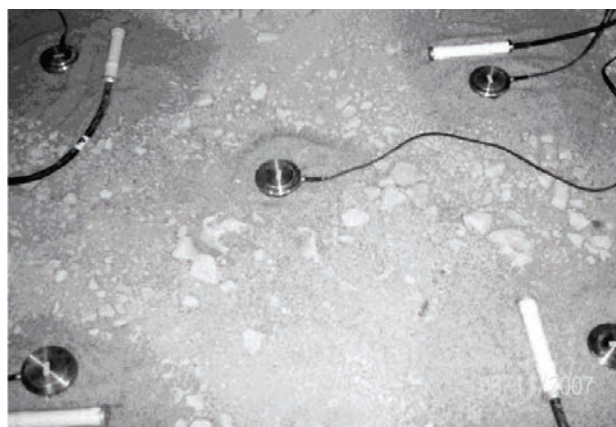
Fig. 5. Pressure gauge and strain gauge placements on top of the subbase layer. Plan view of pressure gauge and and strain gauges
