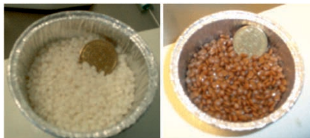
a) b) Fig. 1. WMA additives: a – Sasobit; b – Rediset WMX
