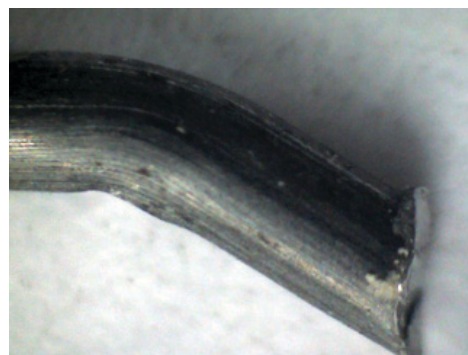
Fig. 2. Magnified (125 times) ending of the steel fibre
