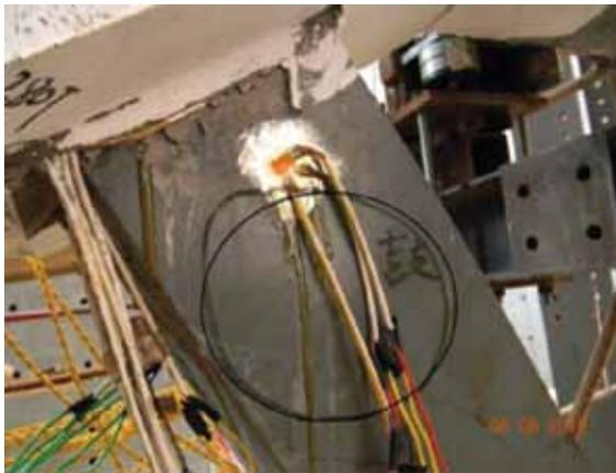
Fig. 7. Buckling of ZHJD-1 compressive web member  $P = 3800$  kN
