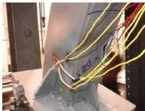
Fig. 9. Failure of ZHJD-2 compressive web member P = 3500 kN
