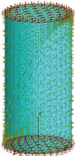
**Fig. 4.** Mesh, boundary and loading conditions for the discrete model of sample
