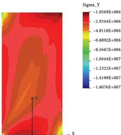
Fig. 9. Distribution of vertical component of stress  $\sigma_y$  in the sample with fixed end
