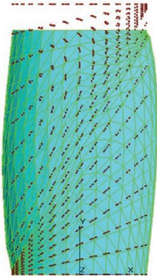
Fig. 11. Deformed shape of sample of triaxial test with fixed ends
