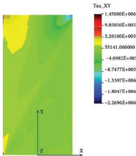
Fig. 6. Distribution of shear stress component  $\tau_{xy}$  in the sample with free ends
