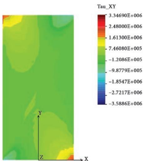
Fig. 5. Distribution of shear stress component  $\tau_{xy}$  in the sample with fixed ends
