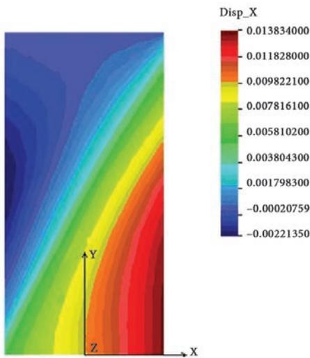
Fig. 8. Distribution of horizontal soil displacements  $u_x$  in the sample with free ends
