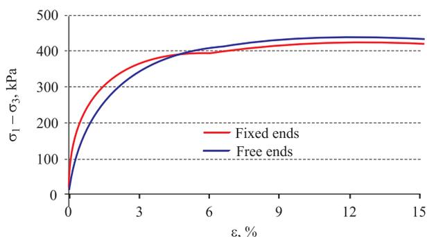
Fig. 3. Stress-strain graph of loose sand, when  $\sigma_3 = 200$  kPa
