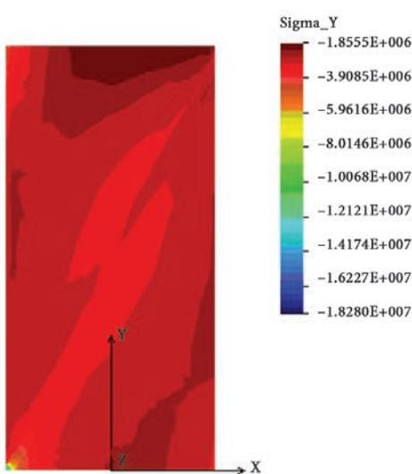
Fig. 10. Distribution of vertical component of stress  $\sigma_y$  in the sample with free ends
