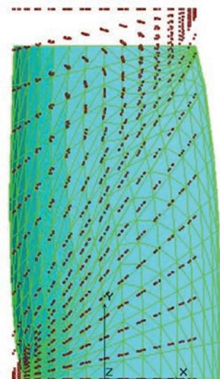
Fig. 12. Deformed shape of sample of triaxial test with fixed ends
