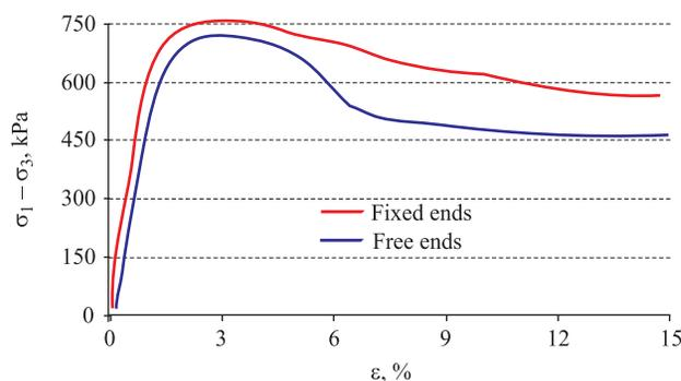
Fig. 2. Stress-strain graph of dense sand, when  $\sigma_3 = 200$  kPa
