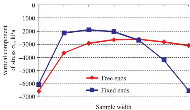
Fig. 13. Distribution of vertical stress component  $\sigma_v$  of specimen base along the section of sample (along X axis)
