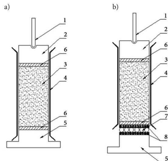
**Fig. 1.** Boundary conditions of samples for triaxial testing: a – with fixed ends; b – with free ends: 1 – rod, 2 – cap (platen), 3 – specimen, 4 – latex membrane, 5 – pedestal (platen), 6 – porous stone, 7 – thrust bearing, 8 – stainless steel plates
