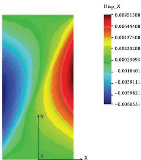
Fig. 7. Distribution of horizontal soil displacements  $u_x$  in the sample with fixed ends
