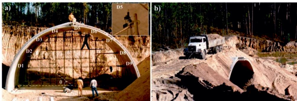
**Fig. 3.** Load test of underpass PA1: a – general view and nomenclature of transducers; b – test in progress
