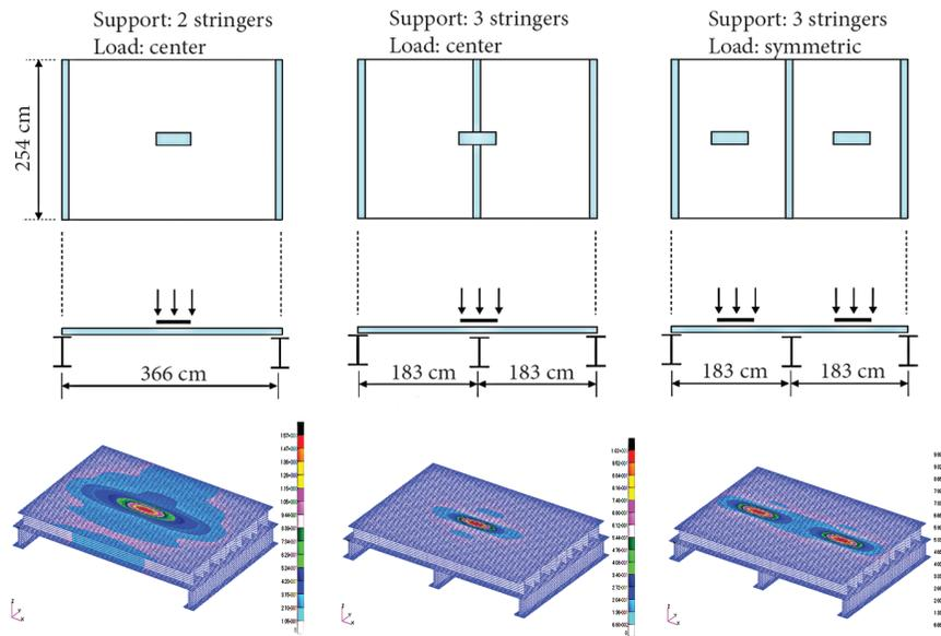
Fig. 4. Finite element models simulated by laboratory experiments
