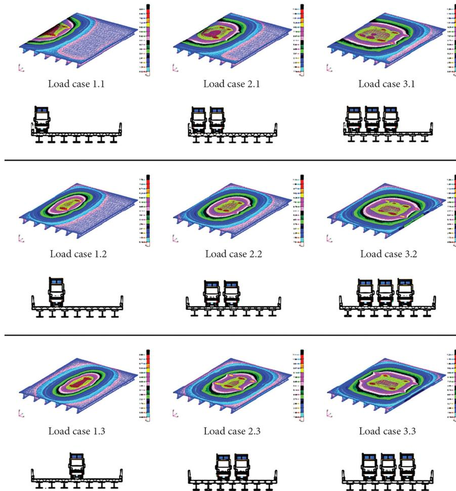
Fig. 5. Finite element models simulated by parametric study
