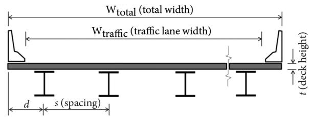
**Fig. 2.** Bridge geometry
