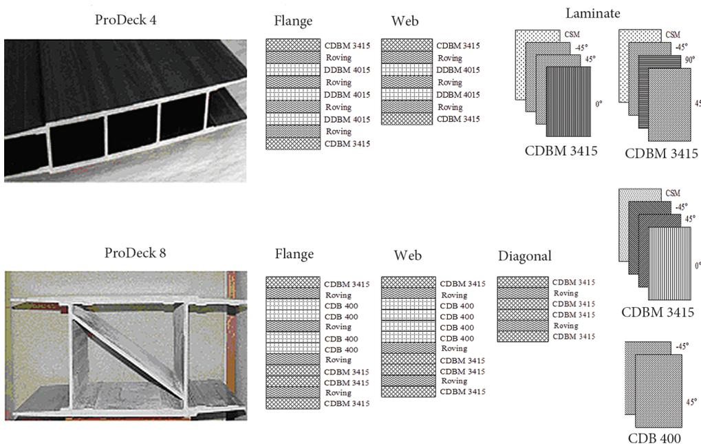
**Fig. 1.** Layer construction and laminate stacking sequence
