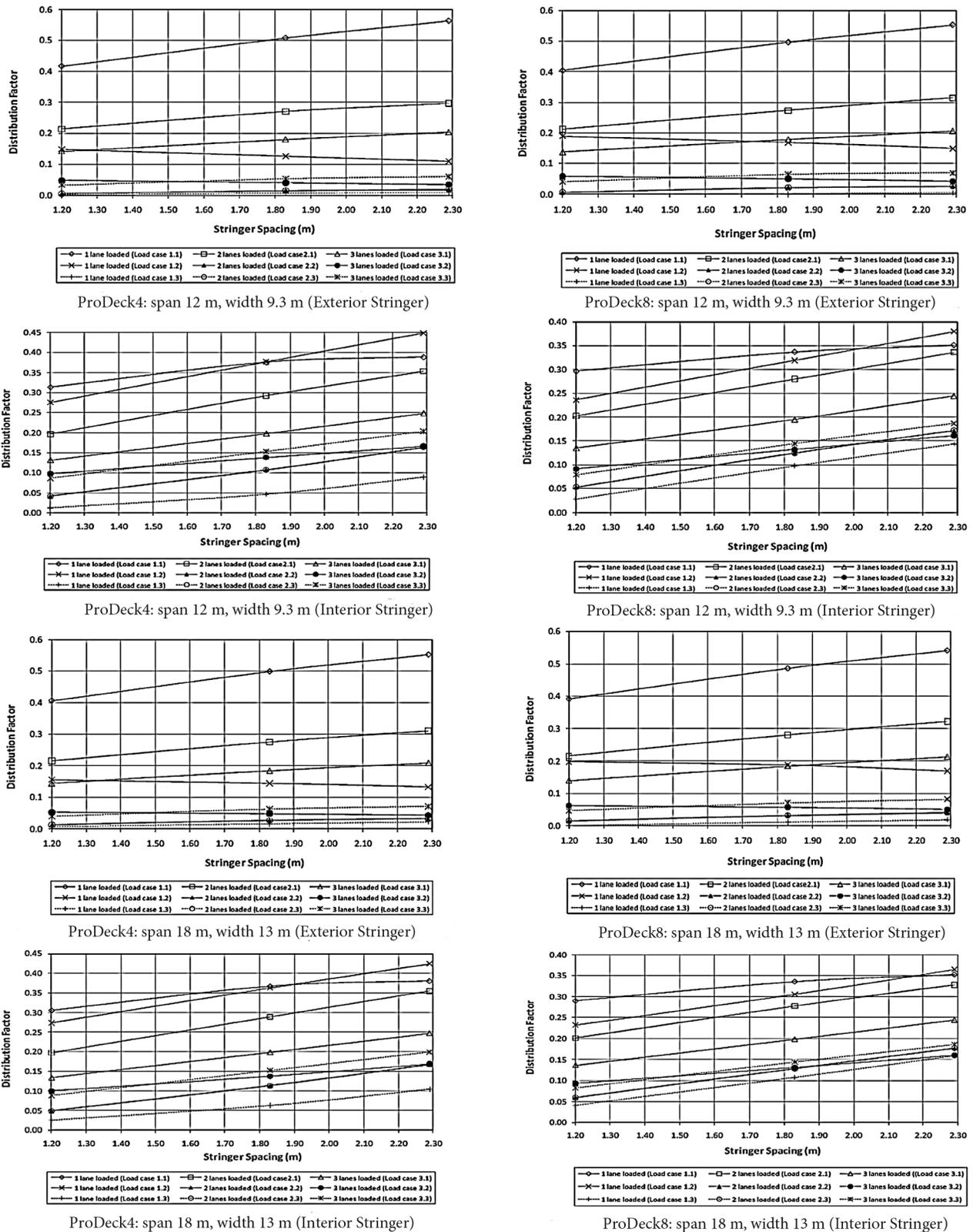
Fig. 6. Load distribution factors for ProDeck 4 and ProDeck 8 – stringer bridge models
