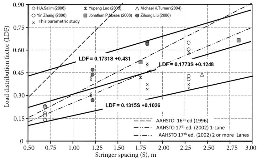
Fig. 7. Comparisons and correlation of load distribution factors with previous data
