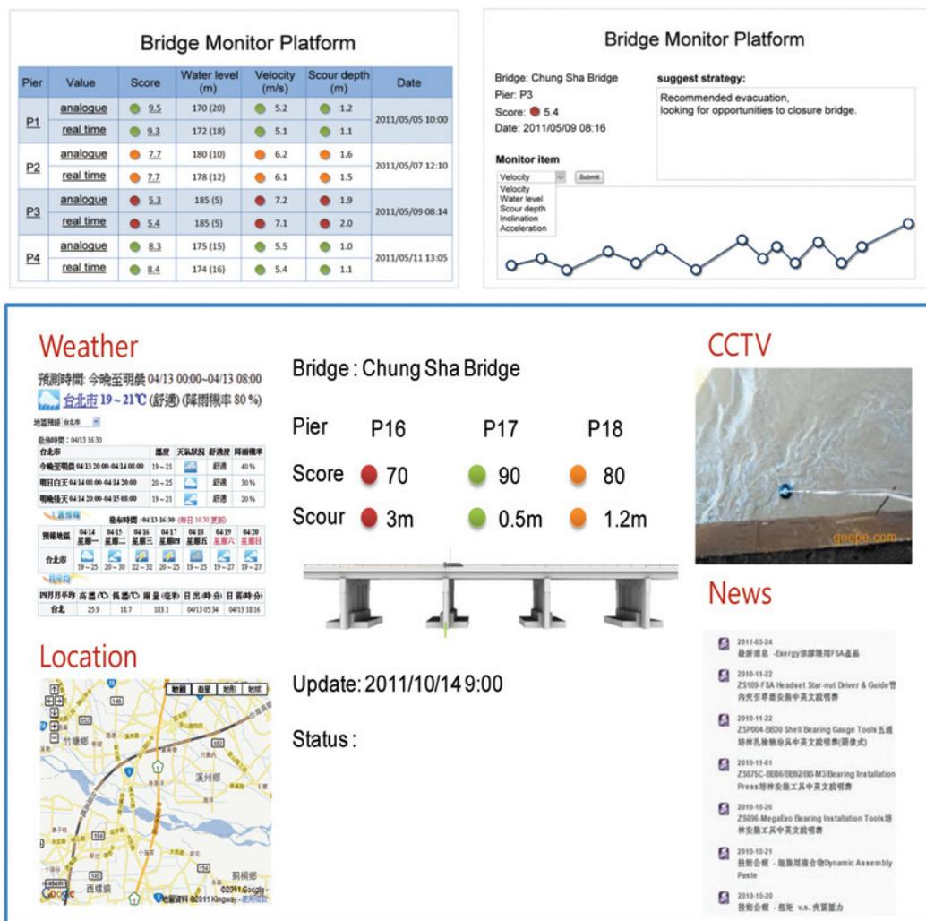
Fig. 8. The platforms of web-based bridge scour monitoring system
