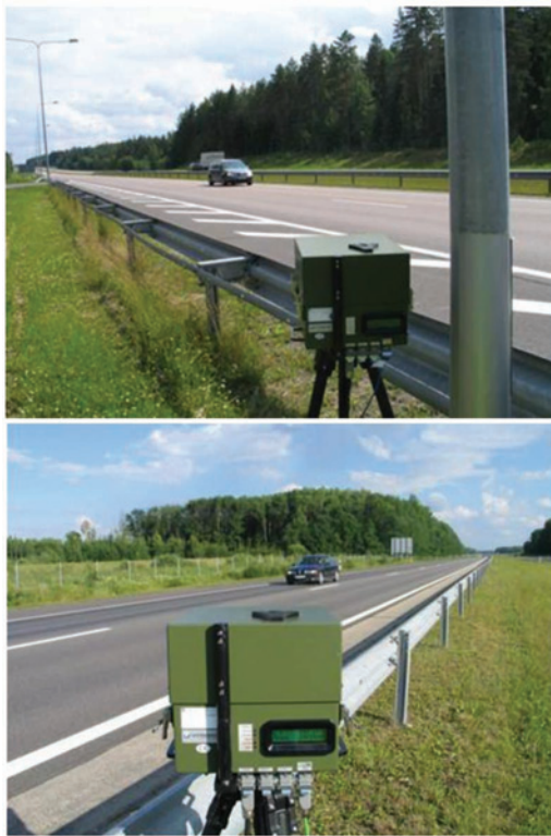
Fig. 2. The sectorial speed enforcement devices on the test section of the road A2 (photo: JSC ATEA)
