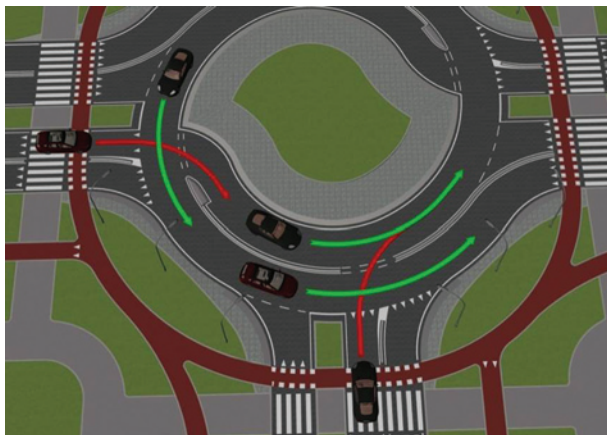
Fig. 9. Crossing conflict spots at the entry onto the inner circulatory carriageway from the inner lane at the entry (designed by Sašo Turnšek)
