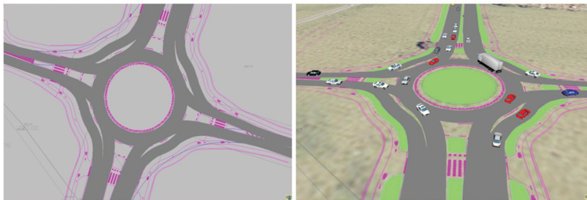
Fig. 11. The mathematical model and 3D simulation of the flower roundabout with PTV Vissim 5.20 (designed by APPIA Ltd. Ljubljana)
