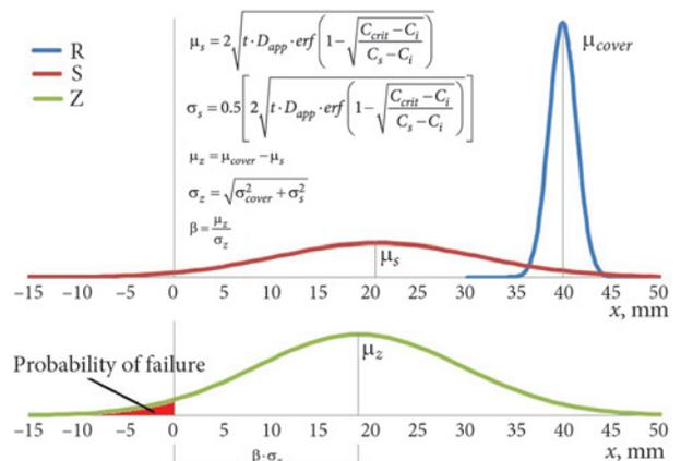
Fig. 21. Reliability concept for performed calculations
