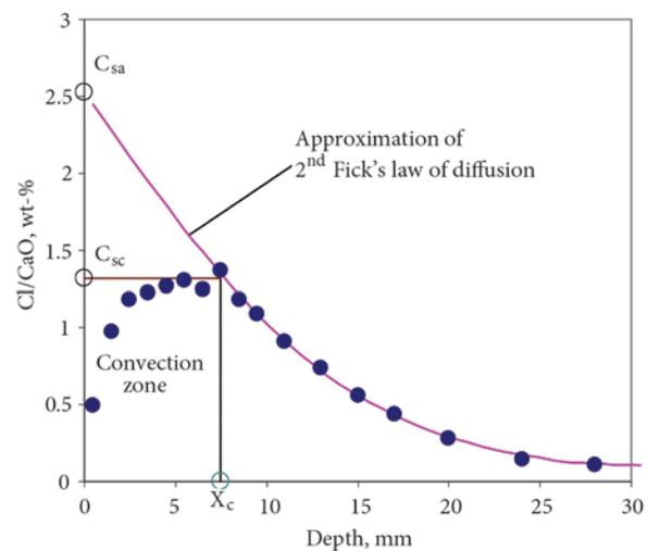
Fig. 1. Chloride profile in the concrete cover (Nilsson 2000)
