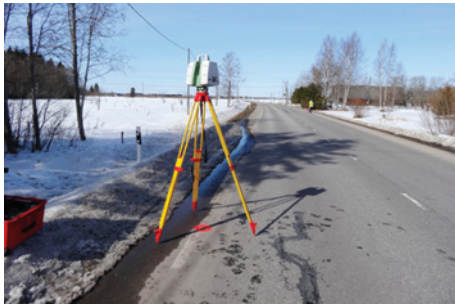
Fig. 5. Scanning the road section A in April 2013. Note thawing snow along road sides
