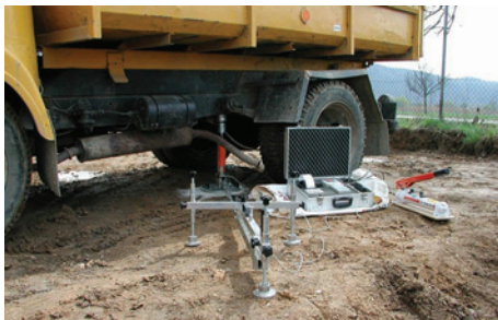
Fig. 1. Static plate loading test
