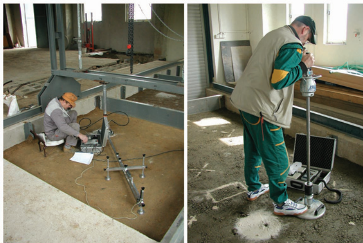
Fig. 7. Tests in the GLTF: static plate test (left) and dynamic LFWD test (right)
