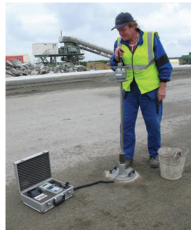
Fig. 3. Dynamic plate loading test using LFWD
