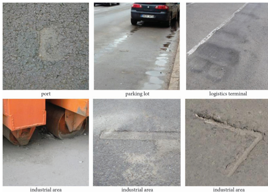
Fig. 1. Examples of permanent deformation observe in pavements of special objects
