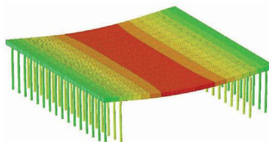
Fig. 6. Spatial numerical model of the piled raft for variant II, general deformable view
