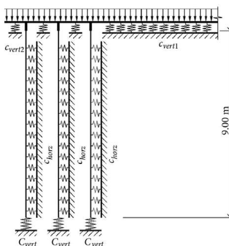
Fig. 3. The soil bed  $c_{vert1}$  and  $c_{vert2}$  stiffnesses of the raft, vertical  $C_{vert}$  and horizontal  $c_{horz}$  spring stiffnesses of the piles
