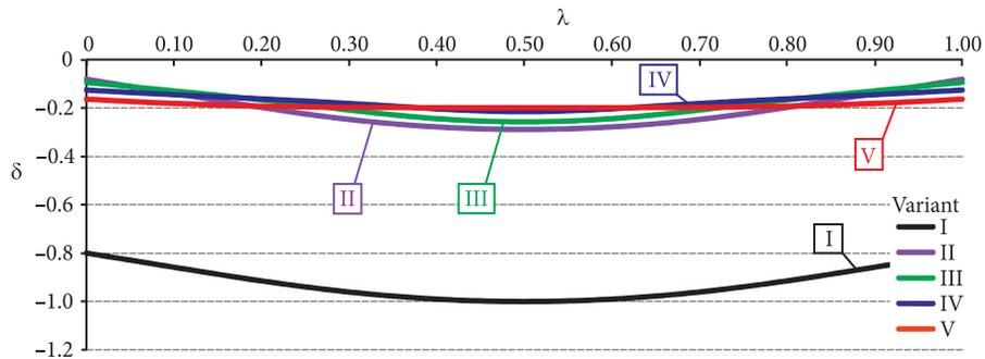
**Fig. 8.** General distribution of relative settlements ( $\delta$ , from 0 to -1) along the raft central axis ( $\lambda$ , from 0 to 1)
