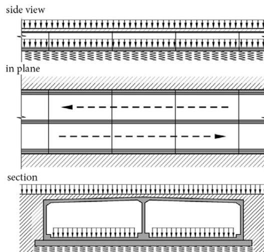
Fig. 1. General views of the road tunnel
