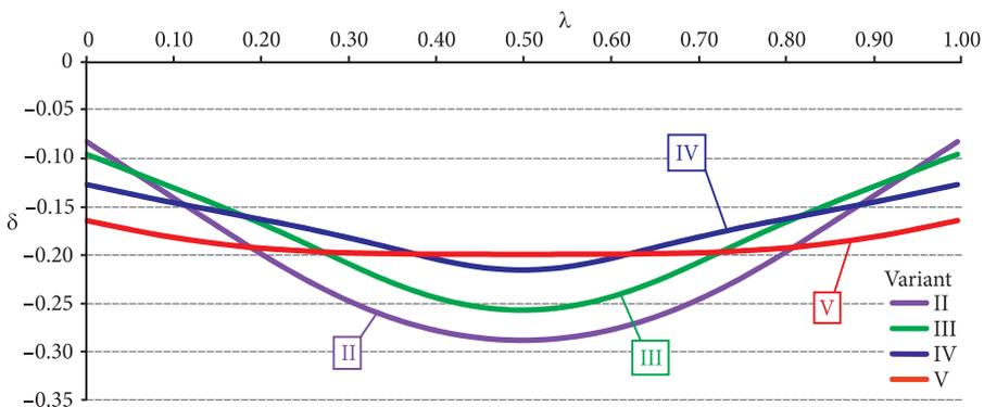
**Fig. 9.** Detailed distribution of relative settlements ( $\delta$ , from 0 to -1) along the raft central axis ( $\lambda$ , from 0 to 1)
