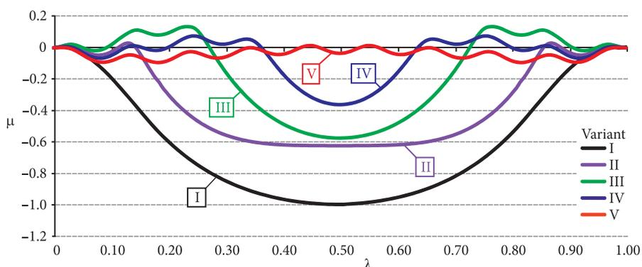
Fig. 10. General distribution of relative bending moments ( $\mu$ , from 0 to  $-1$ ) along the raft central axis ( $\lambda$ , from 0 to 1)
