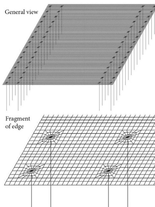
Fig. 5. The spatial numerical model of the piled raft variant II, the finite element grid: general view (a), fragment of edge (b)
