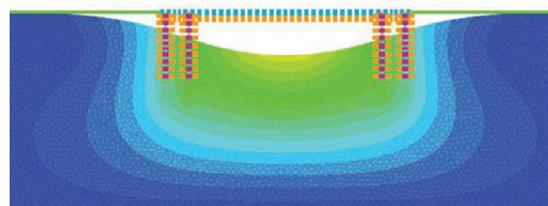
Fig. 7. A deformable view of soil for the piled raft variant II of the plane numerical model
