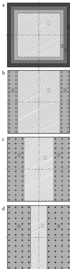
Fig. 4. Distribution of deformable soil bed values: a – unpiled plate; b – 2 and 2 rows; c – 3 and 3 rows; d – 4 and 4 rows
