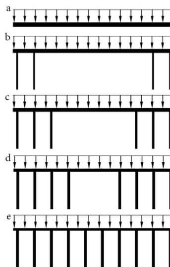
**Fig. 2.** Distribution variants of the raft piles under the raft (in scale): a – unpiled; b – 2 and 2 rows; c – 3 and 3 rows; d – 4 and 4 rows; e – the whole area is piled
