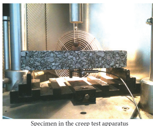
Fig. 3. Bending creep test – the test setup
