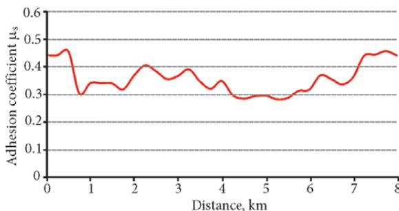
Fig. 7. Changeability of the sliding adhesion coefficient in the measurement points shown on the map in Fig. 6. The mean value of the coefficient equals 0.36
