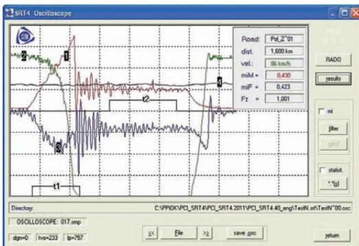
Fig. 3. Exemplary results obtained during braking process (view of the screen): 1 – braking torque  $Wh$ ; 2 – wheel velocity  $\omega$ ; 3 – wheel friction force  $T$ ; 4 – wheel normal load  $F_z$ ;  $t_1$  – time in which  $\mu(s)$  adhesion characteristic is determined;  $t_2$  – time in which average values of friction force are obtained
