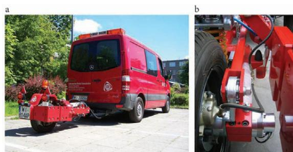
Fig. 1. Measurement system – SRT-4: a – dynamometer trailer and towing vehicle; b – measurement wheel with brake callipers and trailing arms
