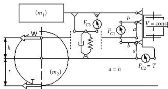
Fig. 2. Kinematic scheme of the dynamometer trailer
