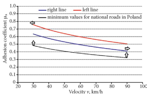
**Fig. 5.** Adhesion coefficient as a function of sliding velocity (see Table 1)
