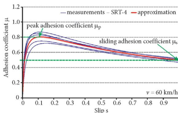
**Fig. 4.** Adhesion characteristics  $\mu(s)$  of one road section: blue – curves obtained for separate points; red – average characteristic
