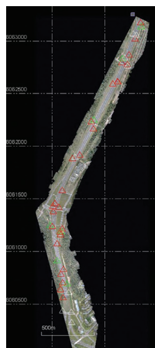
Fig. 5. Distribution of GCPs (marked by white triangles – signalized points, green – check points, red – control points) on the test area
