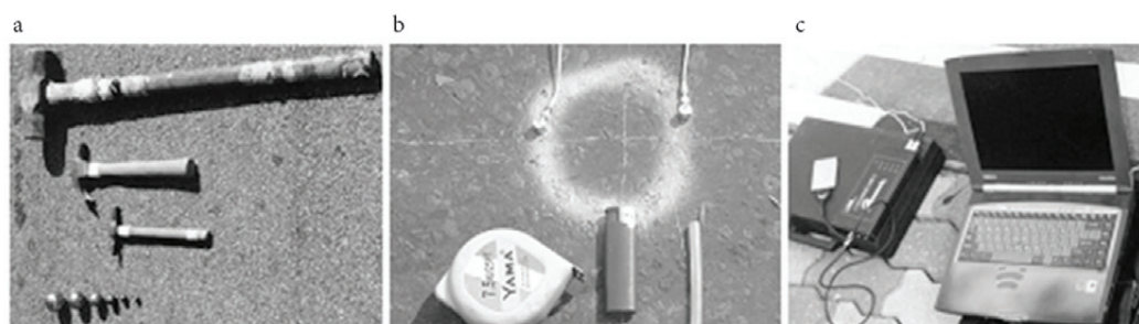
Fig. 2. Instruments used in SASW measurement: a – impact sources; b – accelerometers; c – spectrum analyzer
