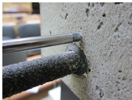
Fig. 3. Slip measurement of BFRP bar at the end of the tested beam
