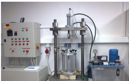
Fig. 4. Apparatus used for triaxial cyclic compression test
