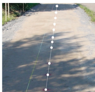
a – deflections obtained by using BB results on an aggregate base course (with corresponding values of moduli of elasticity at subsequent test points located on its surface
