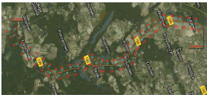
a – example of a road section used in paper (circles mark places where pavement was drilled)
