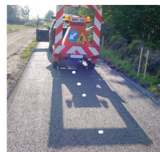
b – an asphalt concrete surface course prepared for deflection tests
