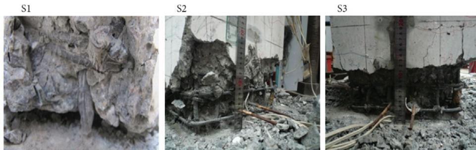
Fig. 11. Failure modes of the specimen columns
