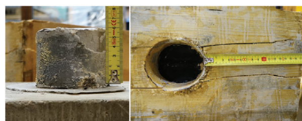
Fig. 12. D76 concrete sample failure (steel intact, wood in compression and shear along the grain)
