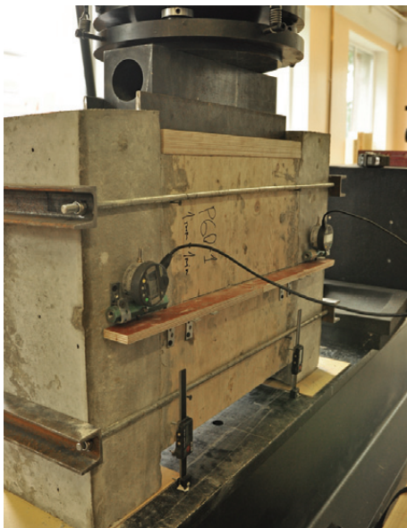
Fig. 6. Laboratory setup of the push-out test
