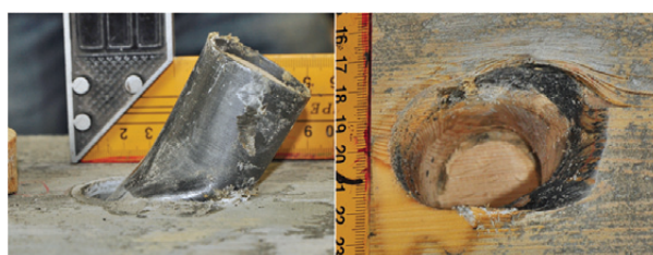
Fig. 9. D42 wood sample failure (steel in shear and wood in compression)
