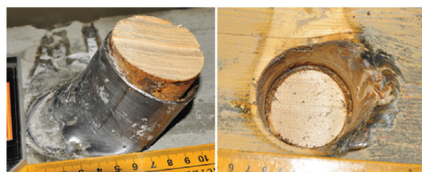
Fig. 10. D60 wood sample failure (steel tearing at extreme slip levels and wood in compression)
