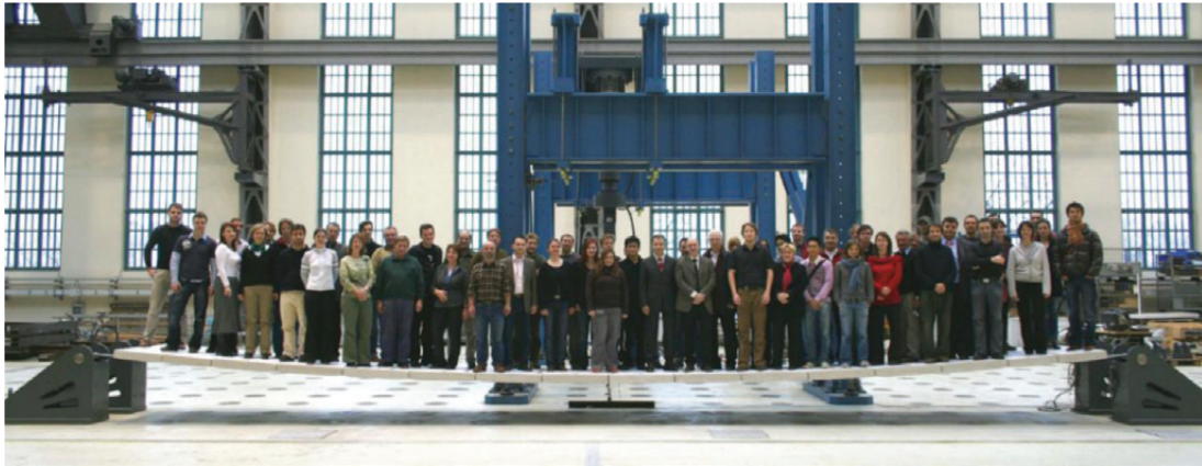
Fig. 1. Load test of the CFRP stress-ribbon bridge (Schlaich, Bleicher 2007)
