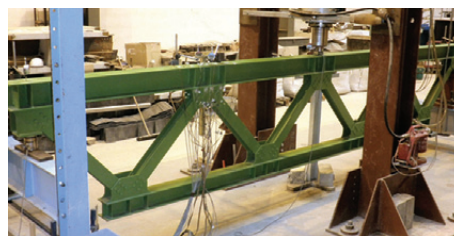
Fig. 13. Tested scaled model of truss girder
