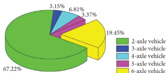
Fig. 4. Proportions of vehicles with different axles
