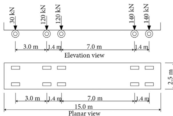
**Fig. 12.** Vehicle model proposed by Chinese code
