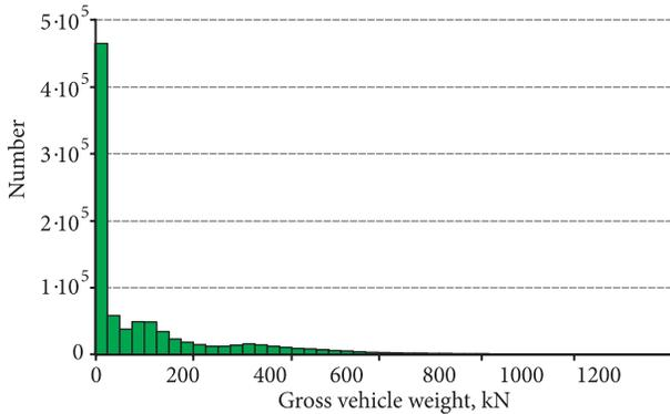
Fig. 7. Statistical histogram of gross vehicle weight
