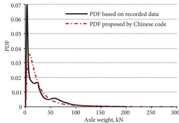
Fig. 10. PDF comparison of axle weight
