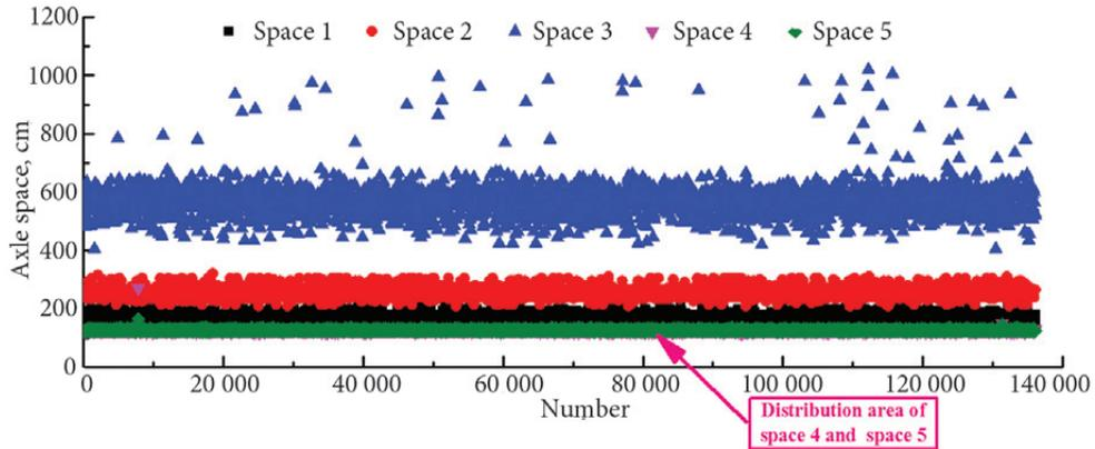
Fig. 14. All axles spacing of 2-1-3 type 6-axle vehicle
