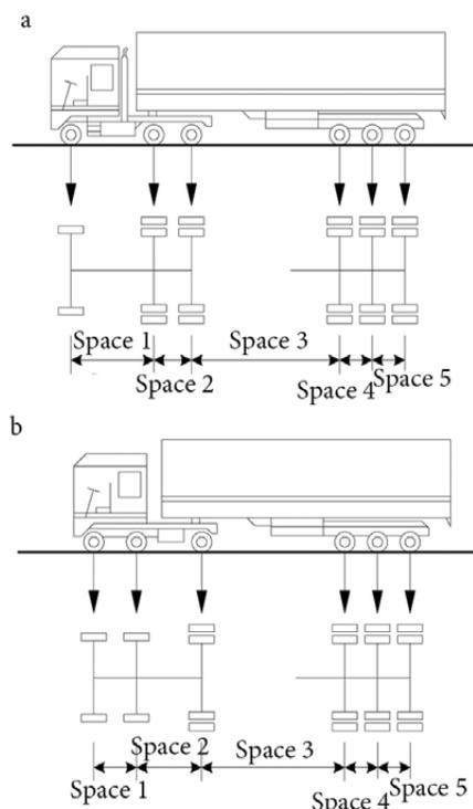
**Fig. 13.** Typical axle-type for 6-axle vehicle: a – 1-2-3 axle type; b – 2-1-3 axle type
