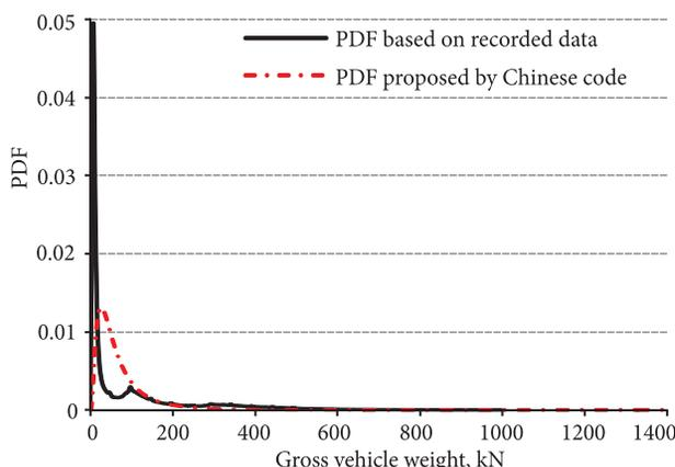
Fig. 5. PDF comparison of gross vehicle weight
