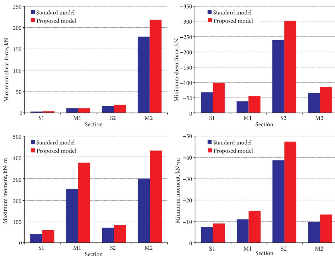
Fig. 16. Comparison of live load effect between code model and measured model
