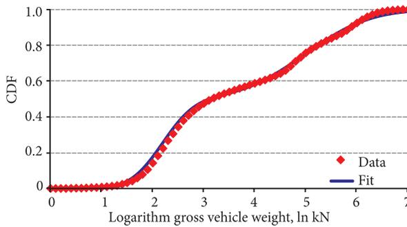
Fig. 9. CDF of the logarithm of gross vehicle weight
