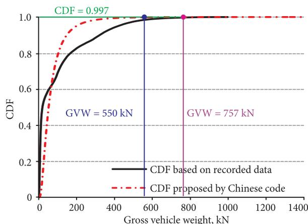
Fig. 6. CDF comparison of gross vehicle weight
