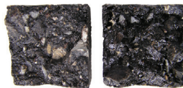
Fig. 9. Fracture surface – binder film thickness difference between mixture I AC 11 (left) and III AC 11 (right)
