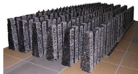
Fig. 3. AC 16 mixtures testing specimens for the determination of stiffness modulus and fatigue characteristics
