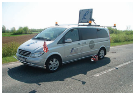
Fig. 2. Measuring vehicle with dynamic retroreflector
