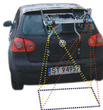
Fig. 3. Measurement vehicle with the stereo vision test-bench
