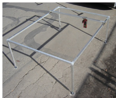
Fig. 5. Reference test-bench with the laser distance meter
