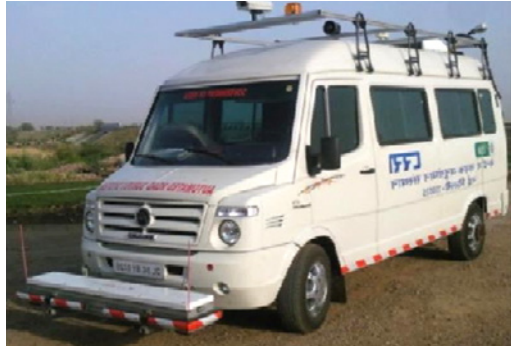
Figure 3. Network survey vehicle with different components
