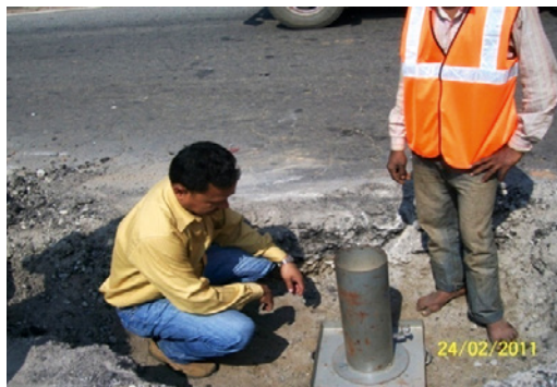
Figure 5. Field density test
