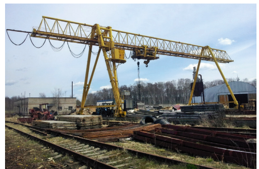
Figure 1. Use of inverted triangular trusses in roof and crane structures: a) roof with the curved inverted triangular trusses (Gusevs, Serdjuks, Artebjakina, Afanasjeva & Goremikins, 2016); b) crane structure with a triangular truss
