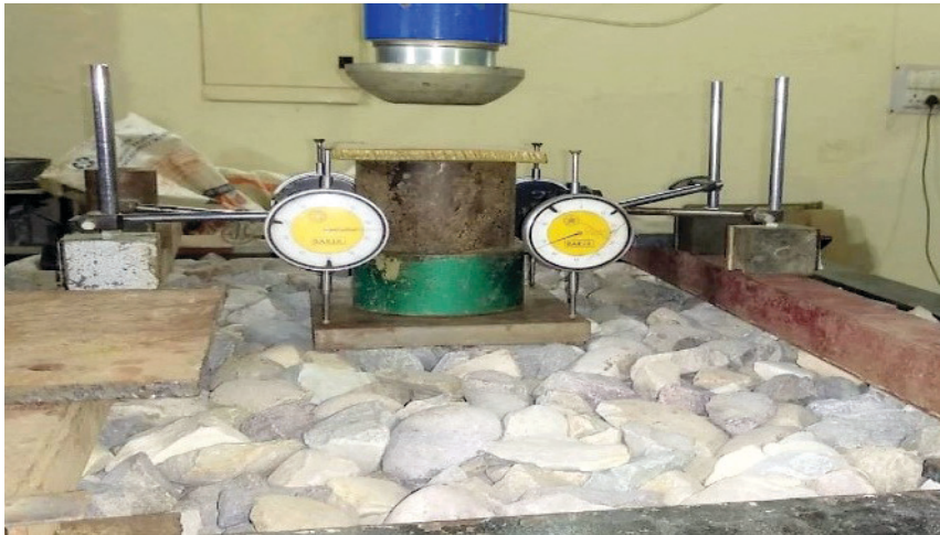
Figure 2. The test setup used in the laboratory showing ballast, dial gauges and loading plate
