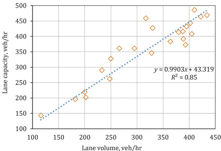
**Figure 5.** The relation between volume ( $v$ ) and capacity ( $c$ ) values on the examined intersection leg lanes
