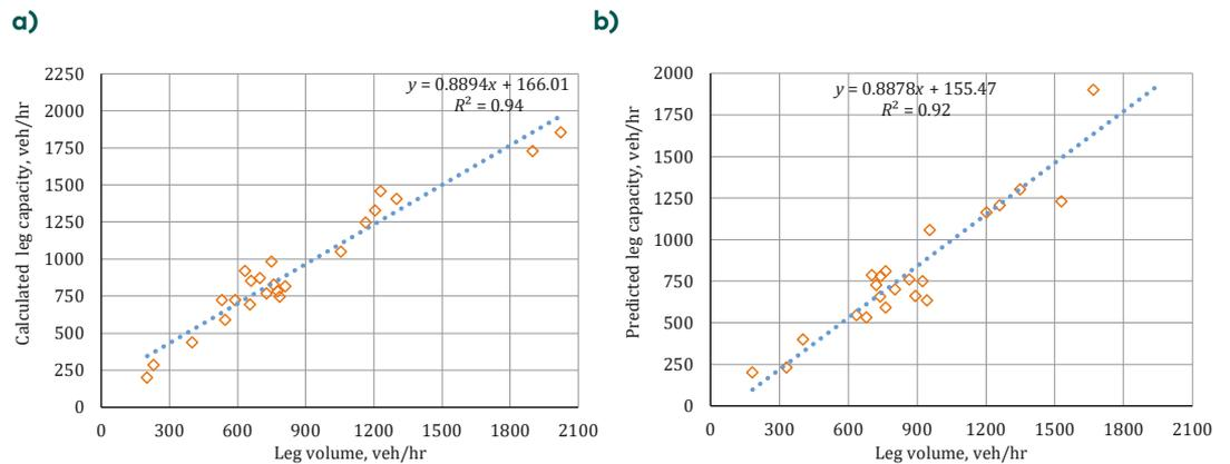
**Figure 8.** Calculated-predicted capacities and volumes for signalized intersection legs
