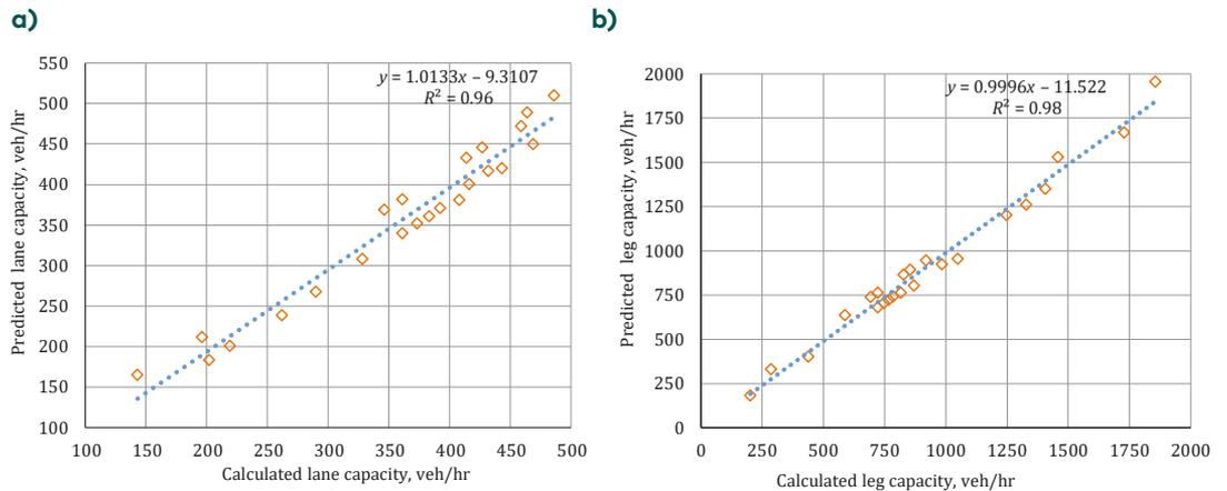
**Figure 7.** The relation between the calculated ( $c_c$ ) and predicted ( $c_p$ ) capacity values for intersection lanes and legs
