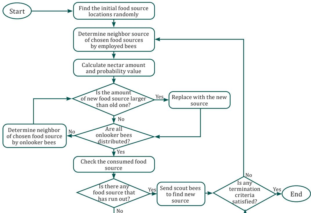
Figure 6. The flow chart of the used ABC algorithm in the model
