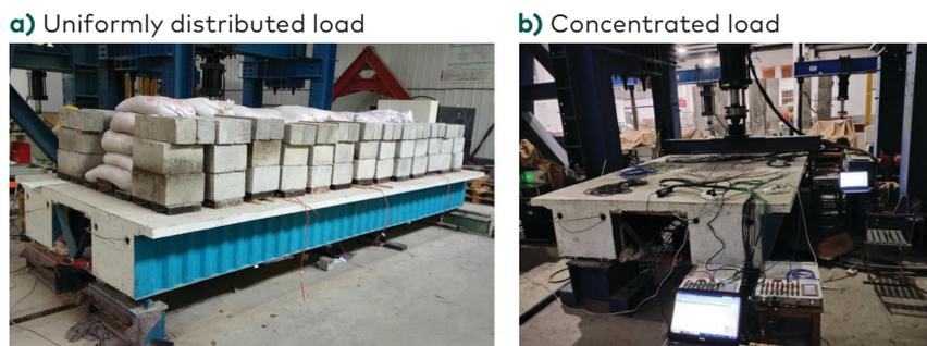
**Figure 5.** Testing load application and mechanical property test
