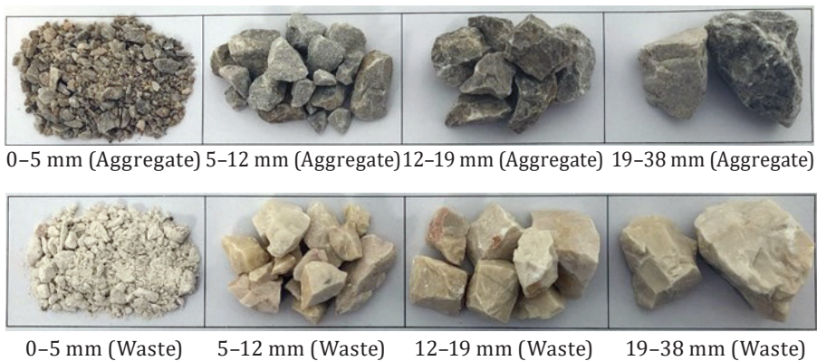
Figure 8. Aggregate and marble waste samples
