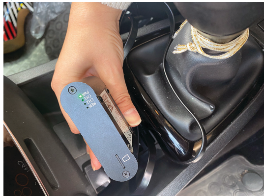
Figure 3. CANedge1 (2x CAN Bus Data Logger) setup and data collection process
